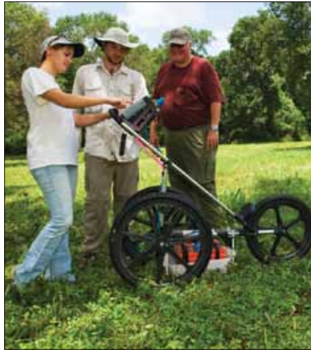
MARKING THE SPOT: Students and instructors search for unmarked graves with a ground-penetrating radar.
